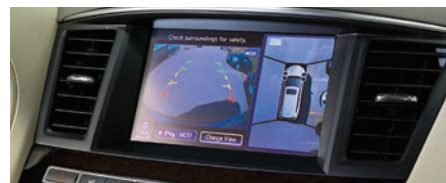
SKY EYE A surround-view camera offers a bird's-eye view of the vehicle when parking.
