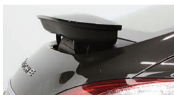
SPEED WING The rear spoiler deploys at 65 mph and retracts at 45.
